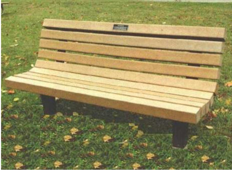
The contoured supports are 3/8" x 4" rolled steel, shaped to provide a smooth, comfortable seat and backrest. The legs are 2- 1/2" square steel support tubing, welded to an arched 3/8" x 4" formed steel base. The frame is coated black for durability and an attractive appearance. The slats are 4" x 4" cedar-color recycled plastic. The bench is mounted directly into the ground, and each leg is anchored with concrete.
